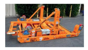
unit, with engine. Tow bar stows on base frame when not in use. Maximum towing speed of unit is 5 km/h (3 MPH). Built-in shock absorbing mounts cushion all transport movements. A series of Tie-down rings (14) offer secure retainment during long distant hauling of unit
