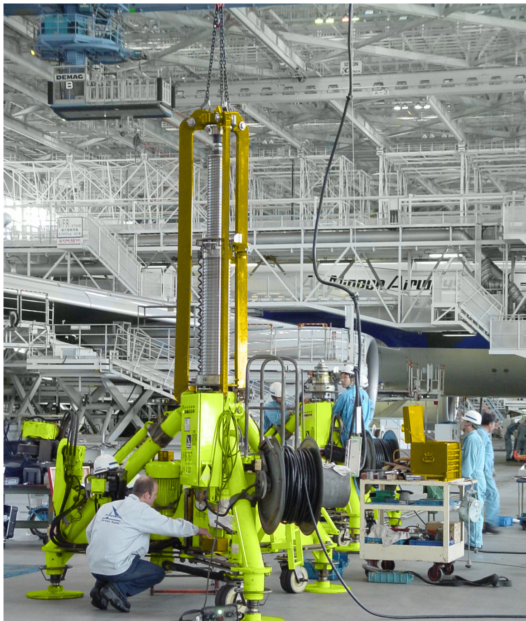
On-site proof load test with HYDRO proof load test fixture PV165
